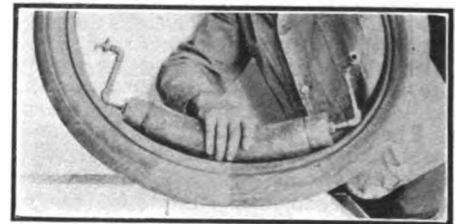
Fig. 8—Twentieth Century Steam Curing Bag for curing the inside of a tire as well as the outside, made by the K. & W. Rubber Co., Denver, Col.
